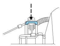
**Note:** If hose clamp is not secured properly or Mass Air Flow Sensor electrical connector is not properly installed the Check Engine light will illuminate when vehicle is operated.
